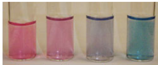
Figure shows the range of colors seen during titration to an endpoint.
