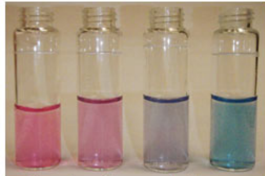
Figure shows the range of colors seen during titration to an endpoint.
